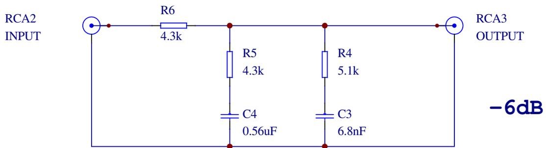
The  $-10\text{dB}$  version is wired up with an XLR at the input and an RCA at the output, while the  $-6\text{dB}$  version is wired up with both RCA at the input and the output. Both versions can be wired up for XLR or RCA input similar to these schematic options. The output, however, needs to be connected to an amplifier input with an impedance of  $47\text{k}\Omega$  or higher. Most RCA inputs will meet that, but most XLR inputs will not.
