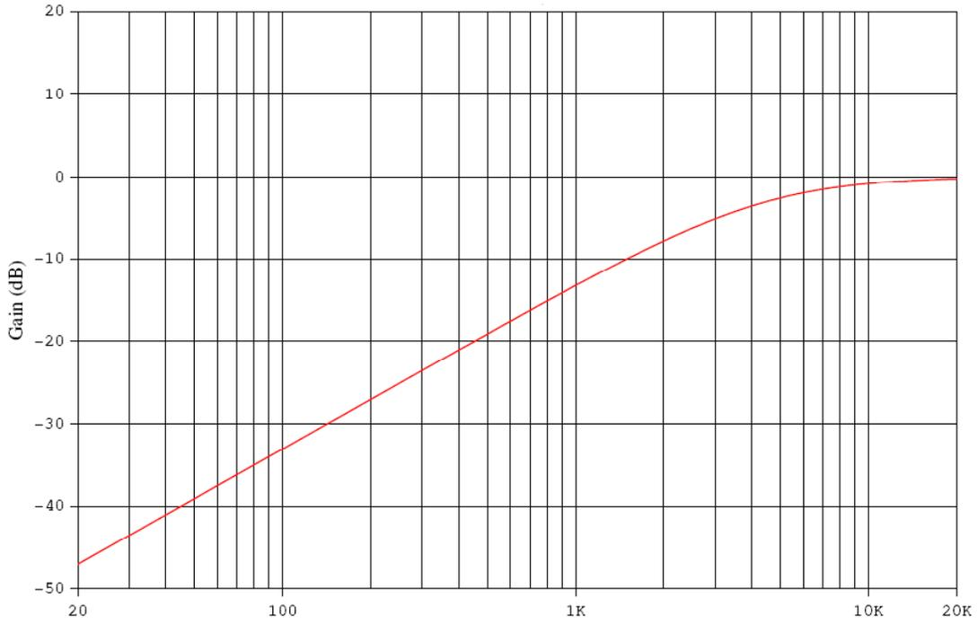
So if we create an inverse frequency characteristic in the playback amplifier like this,
