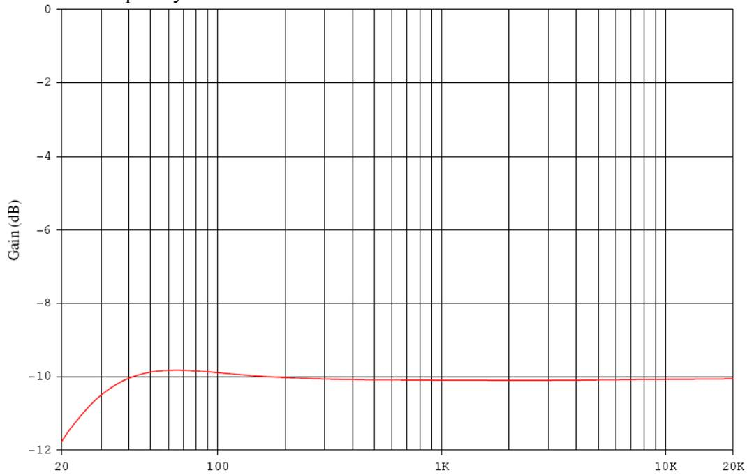
The high frequencies are virtually flat. Certainly much flatter than your tape will ever be. At 30Hz the roll off is less than 0.5dB and it is still less than 2dB at 20Hz.
