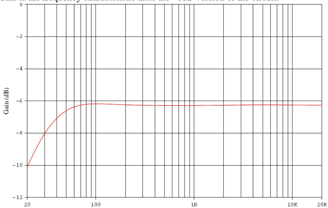
Also here the high frequencies are virtually flat. There is a little more compromise on the low frequency side. At 30Hz the roll off is less than 2dB and at 20Hz it still is less than 4dB.
