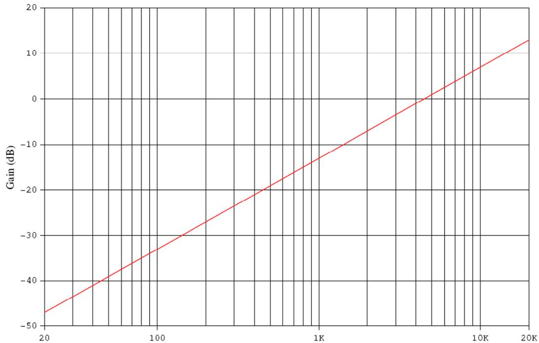
If we add IEC equalization on the recording side, the playback frequency characteristic would look like this:
