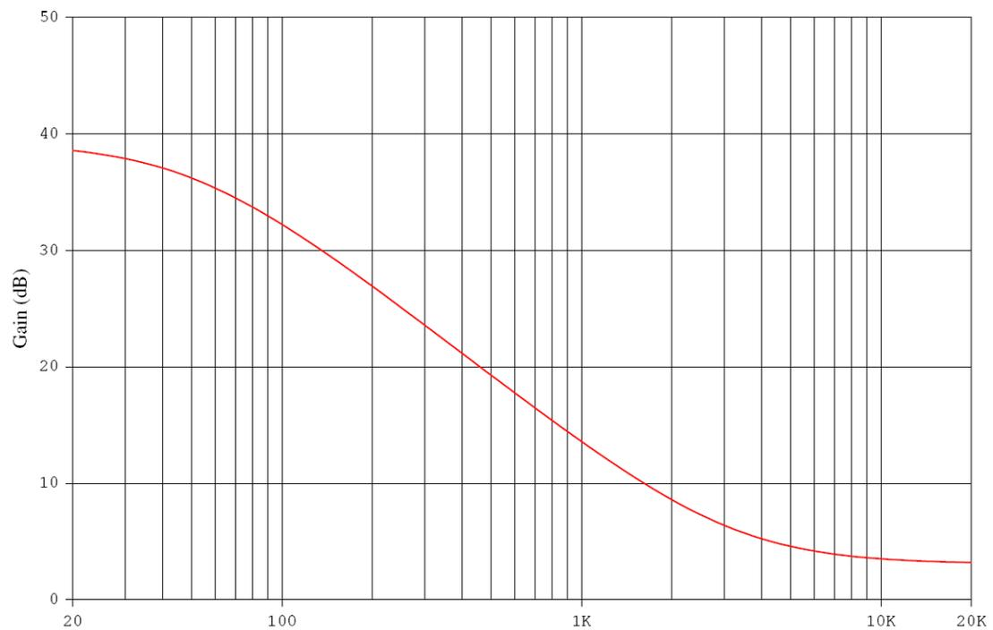
If you combine this NAB equalization on the playback side with a tape that is recorded with IEC equalization, you will end up with this frequency characteristic on the output of your tape recorder.
