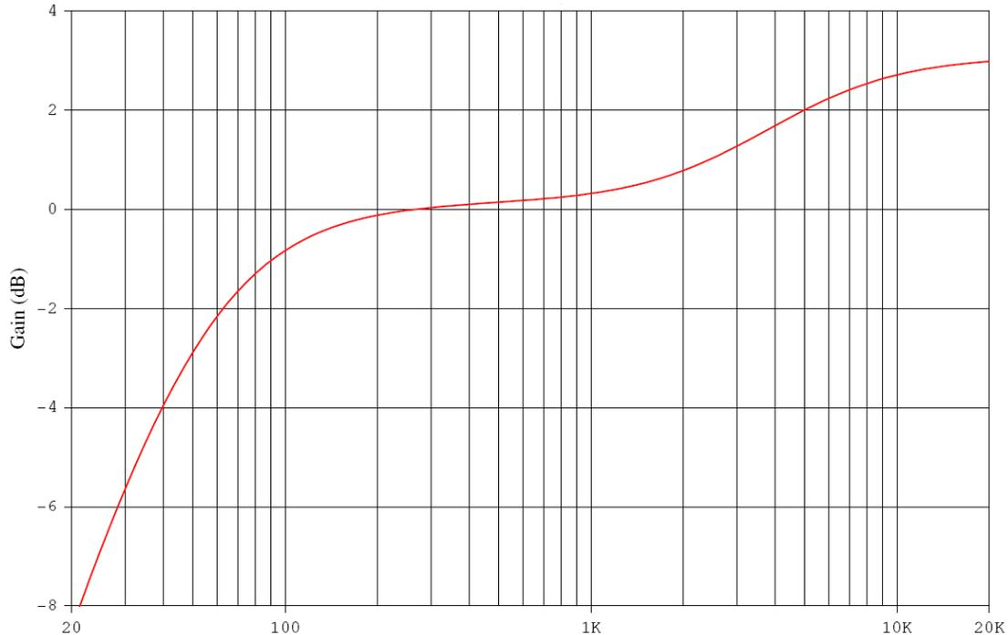
With a lift of 3dB in the higher frequencies the highs will be pretty aggressive and with a roll off of almost 6dB at 30Hz, the bass will be pretty thin.
